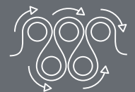
Carding to open and orientate fibres
